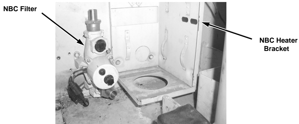
Figure 3-3. New Locations on Driver's Compartment Back Wall.
